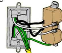
**31** **NEC 250.134** All non-current carrying metal parts of electrical equipment, including raceways, metal boxes and equipment shall be connected to an equipment grounding conductor.
